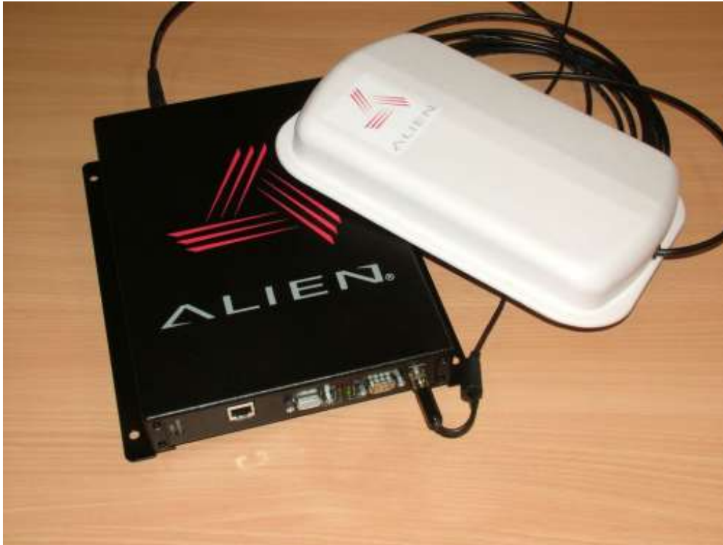
Figure 2. An example of an RFID Reader (black, on left) and aerial (white, on right). Each is about 25 cm x 20 cm. Source: Clayton Jones, Unisys.
